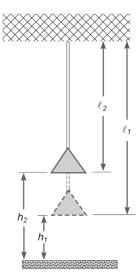
Fig. 3.6 A loaded, constrained rubber band when suddenly released rapidly contracts.
