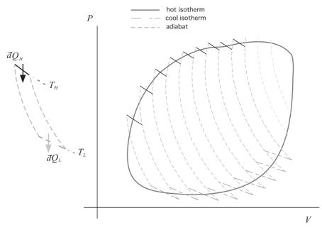
Fig. 4.5 An arbitrary quasi-static (reversible) engine cycle is divided into a series of infinitesimal Carnot cycles, a single one of which is shown on the left.
