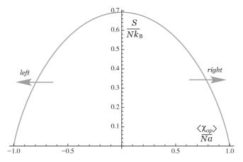
Average extension per monomer,  $\langle \chi_{op} \rangle / Na$ , of an "entropy spring" as a function of S.
