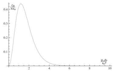
Constant field heat capacity  $C_B/Nk_B$  vs.  $\beta \mu_{\frac{1}{2}} \mathcal{B}_0$ .
