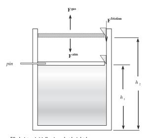
Fig. 3.3 Irreversible work: a gas-filled piston initially pinned at height  $h_1$ .
