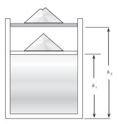
Quasi-static reversible work. A piston loaded down with a pile of fine sand. Fig. 3.1
