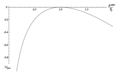
Fig. 3.5 Work  $W_{frict}$  done by the frictional wedge.
