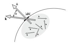
Fig. 14.3 Photon  $\mathbf{k}$  leaving the surface of a radiating body.
