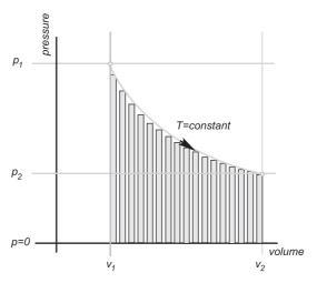
Fig. 3.2 p - V diagram for an isothermal quasi-static process.
