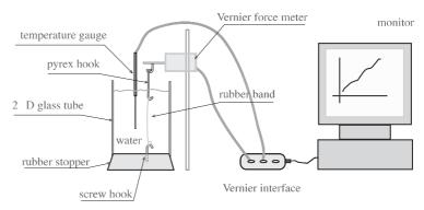
Fig. F.1 Experimental arrangement for measurement of  $\tau$  vs. T. Add boiling water to the glass tube or fill the tube with acetone and dry ice  $\approx -78$  °C. Then allow the system to approach room temperature.
