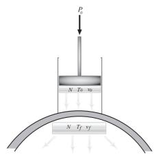
Fig. 3.9 Evacuated vessel filling under pressure  $P_0$ .
