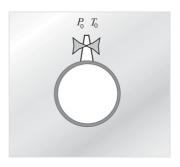
Fig. 3.8 Evacuated, insulated vessel in an atmosphere with pressure  $P_0$  and temperature  $T_0$ .
