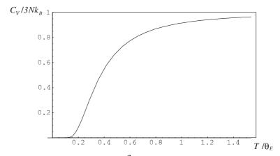
Three-dimensional Einstein model heat capacity  $\frac{C_V}{3Nk_B}$  vs.  $\frac{T}{\theta_E}$ . Note the sharp exponential drop as  $T \to 0$ .
